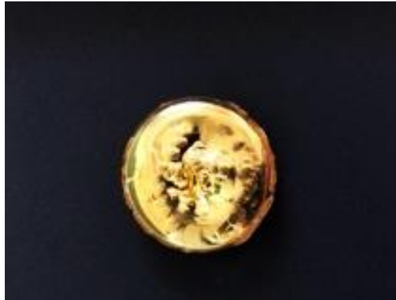
An example of an obtained 50 g Au casting
